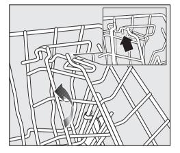
■ Pull the cup rack upwards and click it back into position at the required width.
